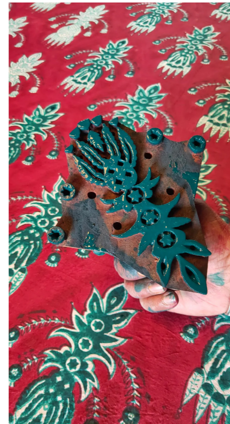
Fig. 2. The process of hand-block printing practiced at 'Jodi'. Source : thejodilife.com
